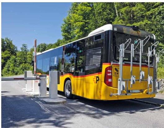
Public transport has also been taken into account: buses pass through the barriers using a special remote-control system.
